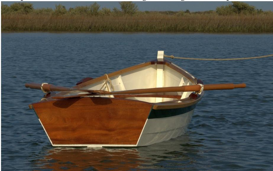
been made in a wide variety of sizes, though typically would measure between 14 and 16 feet long and 4 to 5 feet wide. A larger (up to 38' long) sailing variant of the bateau equipped with a centerboard was known as the sharpie, for its distinctive "sharp" or fine bow. Sharpies evolved in the 1840s from Connecticut oyster skiffs and were introduced to Florida by way of Key West in 1881 and St. Augustine in 1883.
