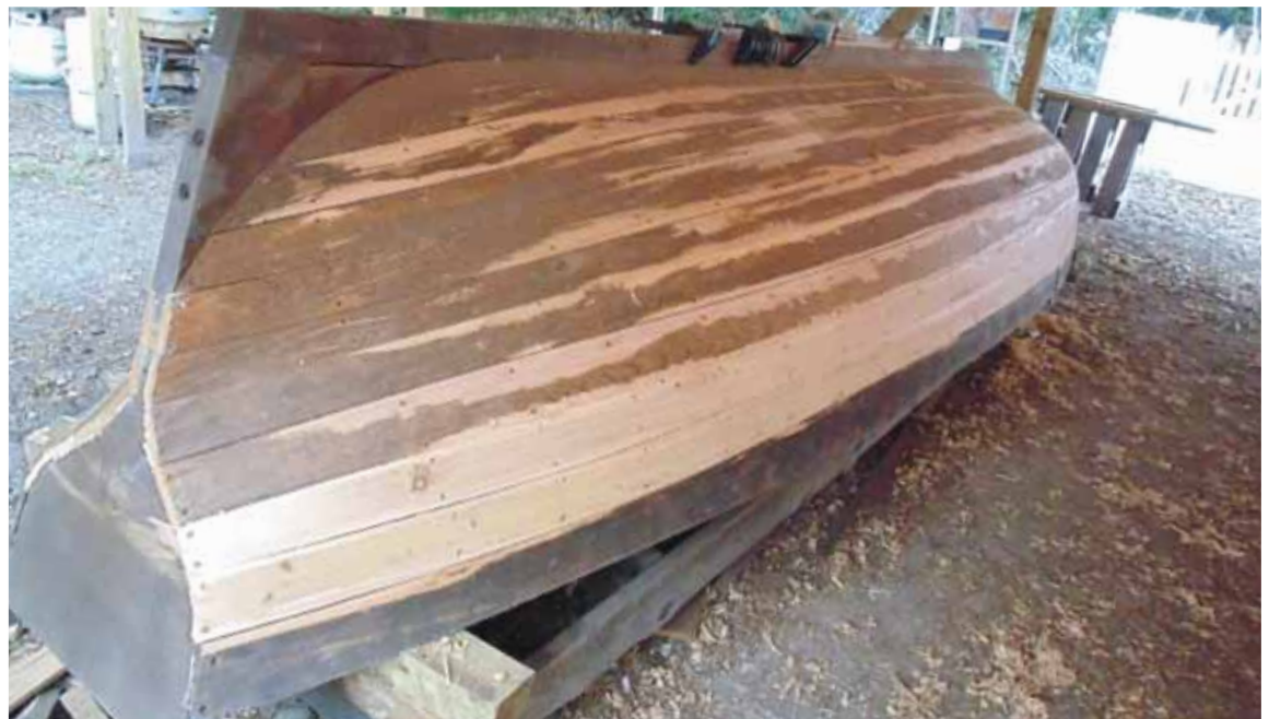
Top: The oak keel and ribs of the yawl boat during its early stages before planking began. Bottom: The cypress planking boards were steamed and bent to the hull of the vessel at the Heritage Boatworks.
