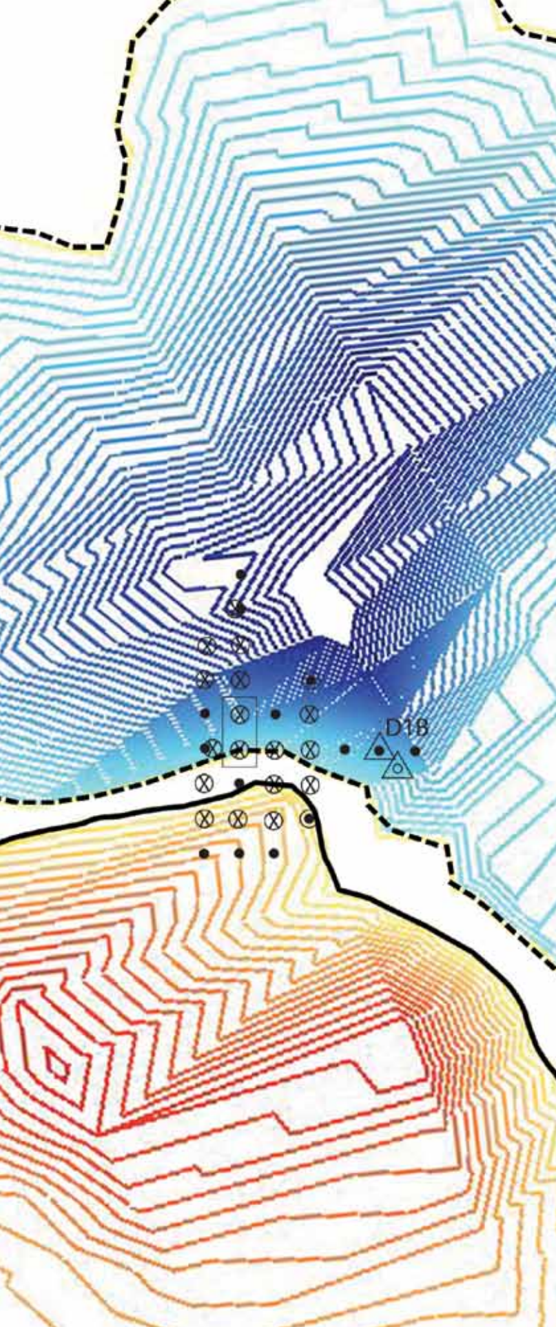
Above, the probe testing sites are laid over the magnetic contour of the Anniversaries Wreck, showing how the data pinpointed the wreck. The X's mark where the probe hit buried objects.
